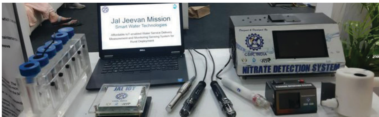
A sensor based IoT device used for assessing and detecting nitrate in water
