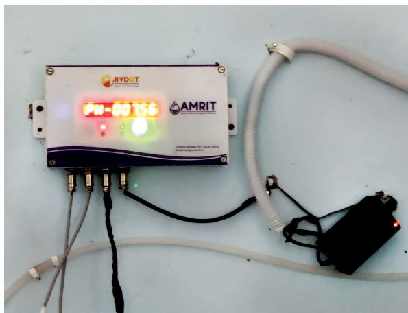
IoT Device for measuring real-time pH of Water supplied
